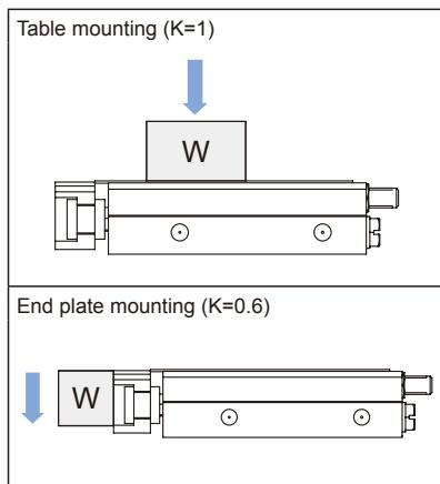
Fig.4: Allowable load mass coefficient:  $\beta$
