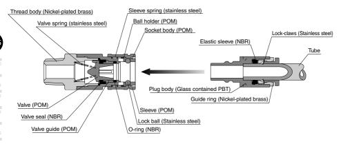
\*\* The above figure is the construction of 15 series. E3 and E7 of 20 series have different construction and materials from 15 series.
