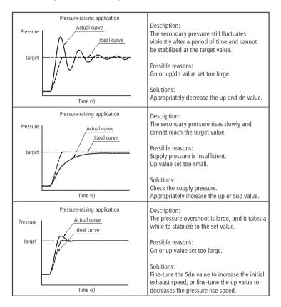
According to different use conditions and occasions, the parameters of the air supply and exhaust valves can be adjusted to ensure that the product meets the needs of use.
