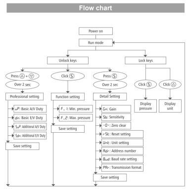
A/V: Air supply solenoid valve ; E/V: Exhaust solenoid valve.
