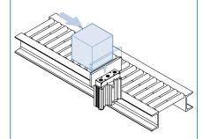
Tough type of stopping a large-load work carrier at a fixed point, and for the straggle of a number of work carriers, etc.
