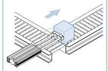
Long strokes available, the highly precise pushing work transfers and places a work carrier and changes the direction.
