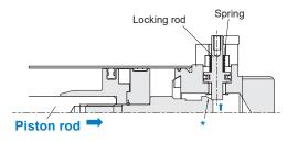
The locking rod will be guided with the slope and keeps moving upward.
