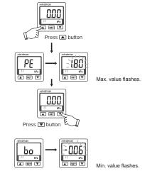
\* This data shows the max. (min.) pressure detected when power supplied
