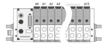
Double coil (007F21 / 007F22) : As shown in the figure below, define the upper coil as  $A0\sim A15$  from left to right; the lower coil as  $B0\sim B15$  from left to right.
